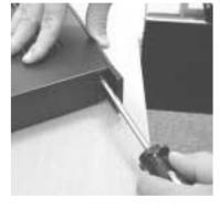
Step Two: Position the rack ears over the threaded holes. Replace the two screws and tighten both securely.
